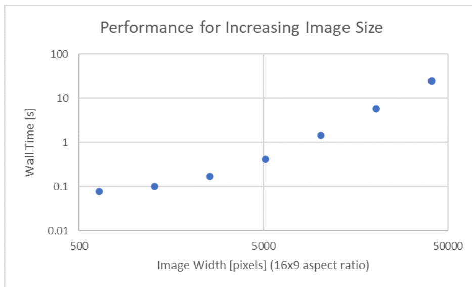
Figure 3.8: Scaling of a single camera shows the performance impact of increasing image size. Configuration: 16x9 camera aspect ratio, 30 Hz update frequency, 10 seconds of simulation time, 173k triangle scene, RTX 2080ti GPU.
